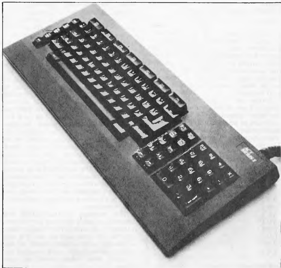
Slimline remote keyboard is IBM Selectric format
